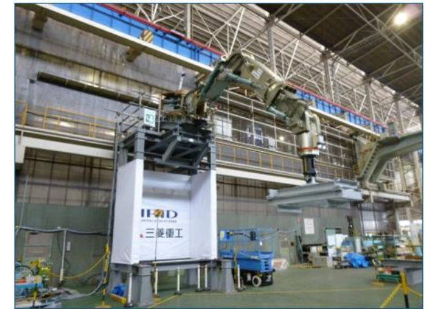
Rendering of Mitsubishi Heavy Industries' seven-meter-long robotic arm capable of withstanding up to 2000 kg of processing reaction force
