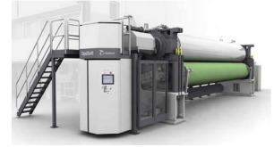
Papermaking equipment. The machine's calender is controlled by a digital hydraulic system.
